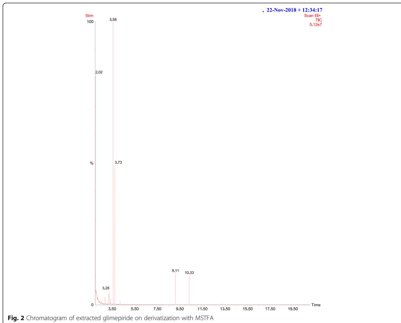
monitoring the analytes at  $m/z$  256 for glimepiride through GC-MS analysis. Hence, the proposed method is specific.
