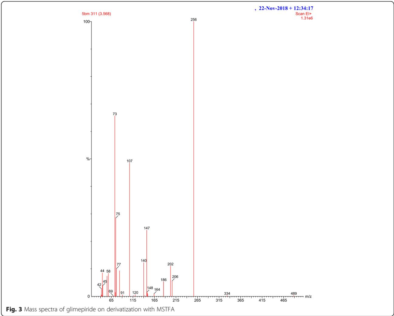
Fig. 3 Mass spectra of glimepiride on derivatization with MSTFA
