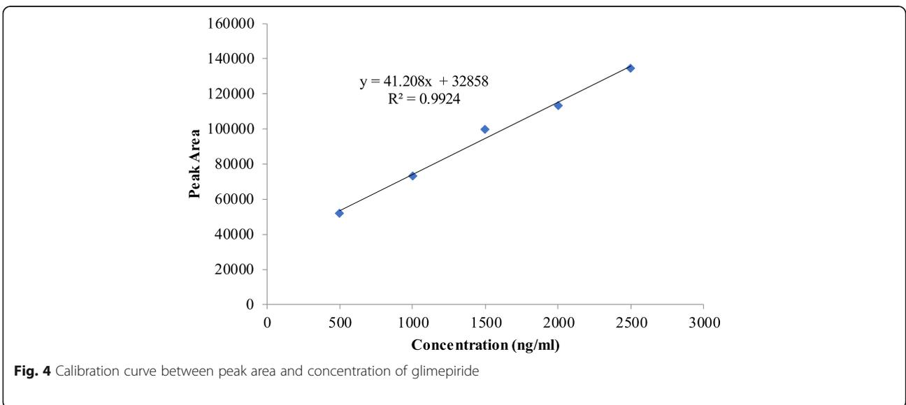
Fig. 4 Calibration curve between peak area and concentration of glimepiride
