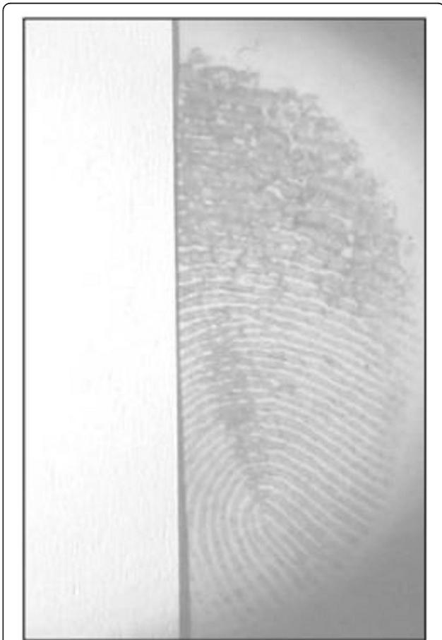
**Fig. 2** Example of fingerprints on thermal paper developed with LED torch (adapted from Bond (2015b))
