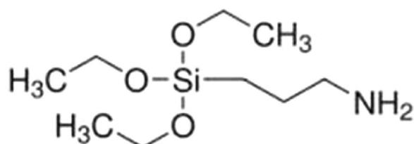
**Fig. 8** Structure of 3-aminopropyltriethoxysilane
