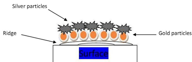
**Fig. 6** Mechanism of multimetal deposition technique
