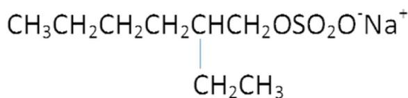
**Fig. 7** Structure of 2-ethylhexylsulfate
