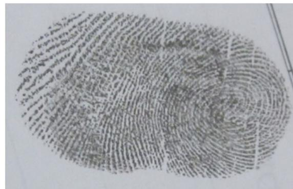
**Fig. 9** A fingerprint developed by multimetal deposition technique
