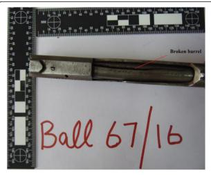
Fig. 2 Showing broken barrel of country made pistol (India)
