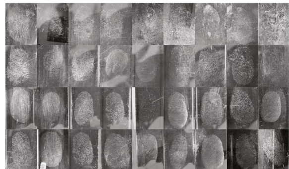
Fig. 5 Fingermarks developed using WP from 36 different donors of various age, sex and race. Compared to the SNP-developed fingermark, WP produces higher contrast in the developed marks; however, overpowdering can be observed along the ridge lines
