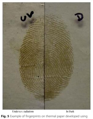
Fig. 5 Example of fingerprints on thermal paper developed using iodine fuming observed under UV light (left panel), and in dark (right panel)
