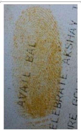
**Fig. 3** Example of fingerprints on thermal paper developed with turmeric powder (adapted from Garg et al. (2011))
