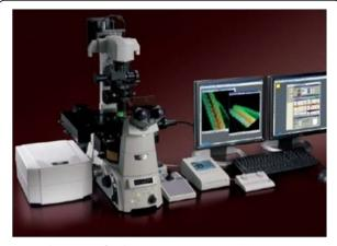
Fig. 1 Nikon A1 confocal microscope
