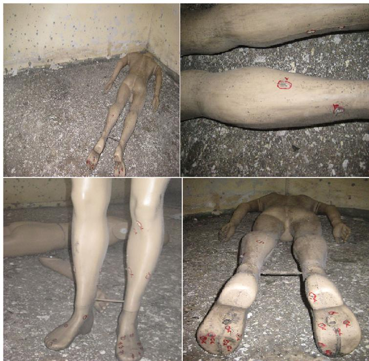
**Fig. 14** Mannequin-2 (male-2) lied face down on left opposite corner after detonation
