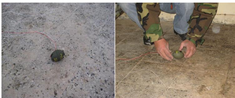
**Fig. 10** The two DM-41 hand grenades primed in for test detonation
