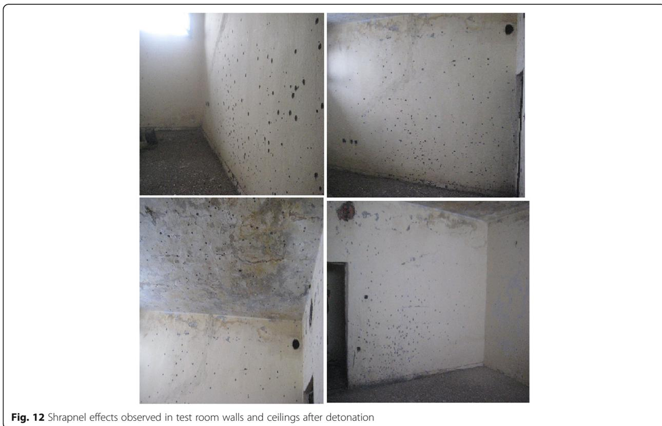
**Fig. 12** Shrapnel effects observed in test room walls and ceilings after detonation
