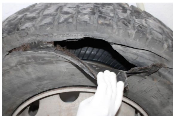
Fig. 1 A zipper-like appearance burst of the upper sidewall area of the tyre
