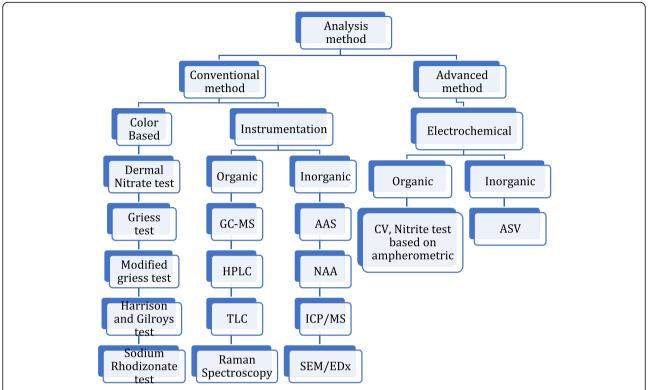
**Fig. 3** Flowchart showing schematic diagrammatic representation of various developed method to detect GSR. ASV, abrasive stripping voltammetry; SEM/Edx, scanning electron microscopy/energy dispersive X-ray analysis; CV, cyclic voltammetry; ICP/MS, inductively coupled plasma mass spectrometry; TLC, thin-layer chromatography; NAA, neutron activation analysis; AAS, atomic absorbance spectrometry; GC-MS, gas chromatography-mass spectroscopy; HPLC, high-pressure liquid chromatography
