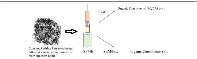
Fig. 4 Gunshot residue analysis technique using solid-phase micro extraction. SPME, Solid-phase microextraction; EC, ethyl centralite; DPA, diphenyl amine
