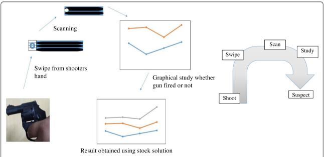
Fig. 6 Sequence of GSR analysis using ASV "Swipe and Scan" method. The Arrow Figure shows the Abrasive Stripping Voltammetry simplified method where firearm shoot, and Gunshot Particles were Swiped, Scanned and then studied whether firearm discharged or not
