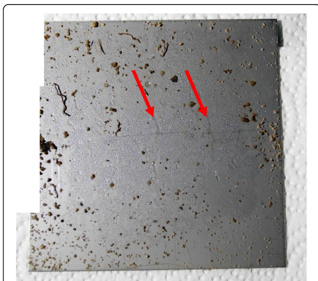
Fig. 13 The formation of water speckles on metal plates bearing the fingermarks (“face down”)
